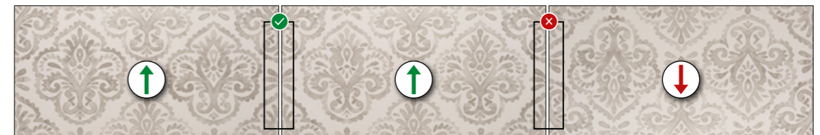
example of correct and incorrect alignment
