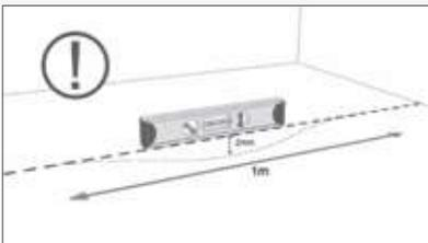
It shall not have defects in its flatness larger than 2 mm, checked using a 2 m ruler.
