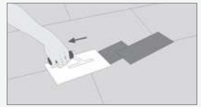
The grouting material is applied with a hard rubber trowel, passing it repeatedly crosswise over the joints.
