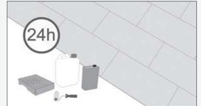
This process shall be carried out 24 hours after the protection of the stones (step 4).
