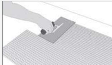
The adhesive is applied with an adequate-sized notched trowel depending on the format of the piece to install.
