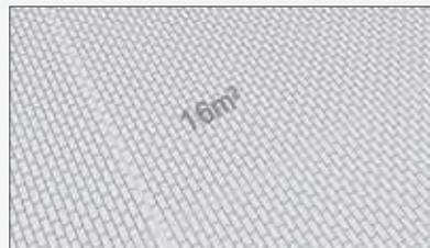
Both perimeter and expansion joints shall be 10 mm wide, and we shall not leave a surface area greater than 16 m<sup>2</sup> or 8 m without an expansion joint.
